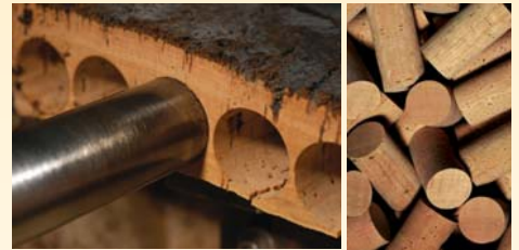
Composite cork coasters are produced from the remnants of wine cork production
